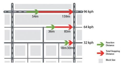
Note: Assumes 2 seconds reaction time and vehicle deceleration rate of 3.4 m/s<sup>a</sup>.
