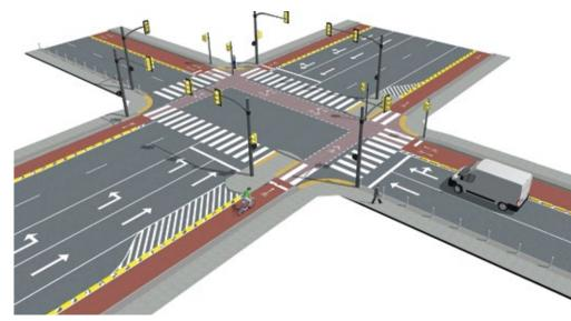
Cycle tracks separated from car traffic through physical barrier.
