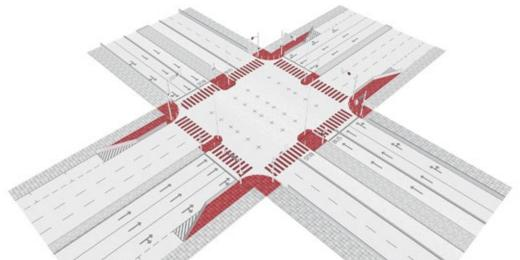
Providing curb extensions and median refuges decrease crossing distance and reduce exposure to moving vehicle traffic.
