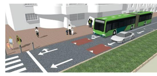
Speed cushions can allow wide-axle vehicles to pass over the cushion to increase comfort for bus passengers.
