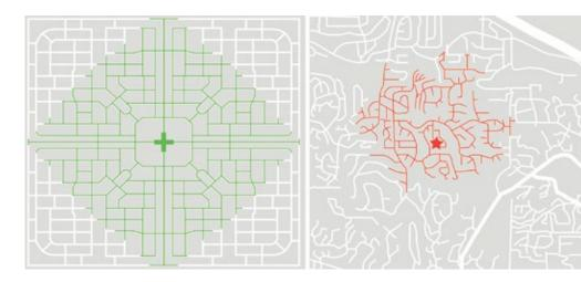
Comparison in 800-meter radius walking catchment in different street connectivity scenarios (compact grid vs. sprawling suburb).
